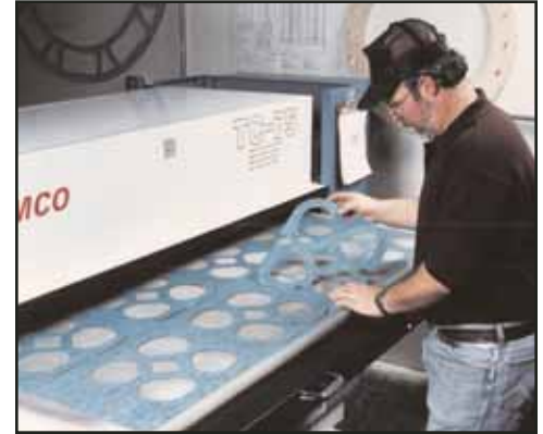
Kenneth's full-beam cutting presses provide increased versatility for fabricating gaskets of various sizes.
